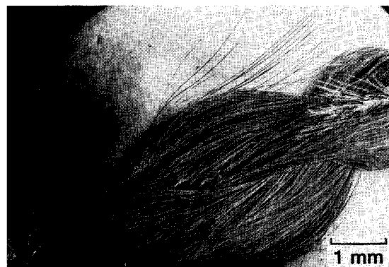
Fig. 6 Nextel 440 fiber-pin specimen after sliding for 24 h at 25°C. Very few fibers are broken, indicating good durability.
