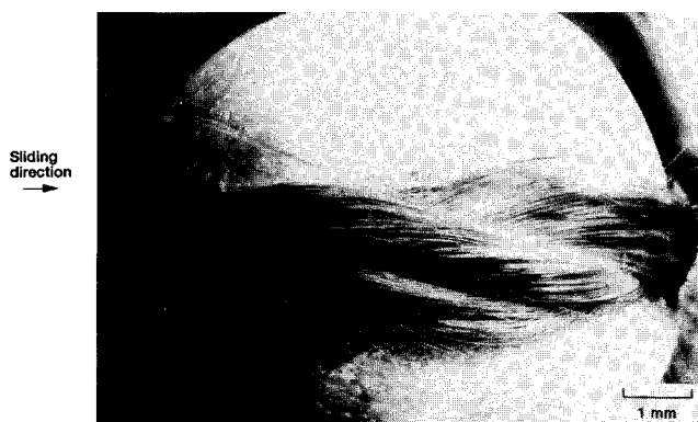
Fig. 3 SEM photomicrograph of fiber-pin specimen prior to testing. Sliding direction is from left to right.
